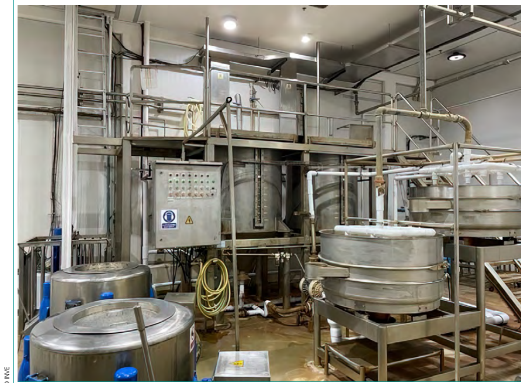
PLATE 39 Example of standard equipment items in cyst processing: Centrifuges (left, front); sets of sieves (right, front); tanks for freshwater density separation (back)
