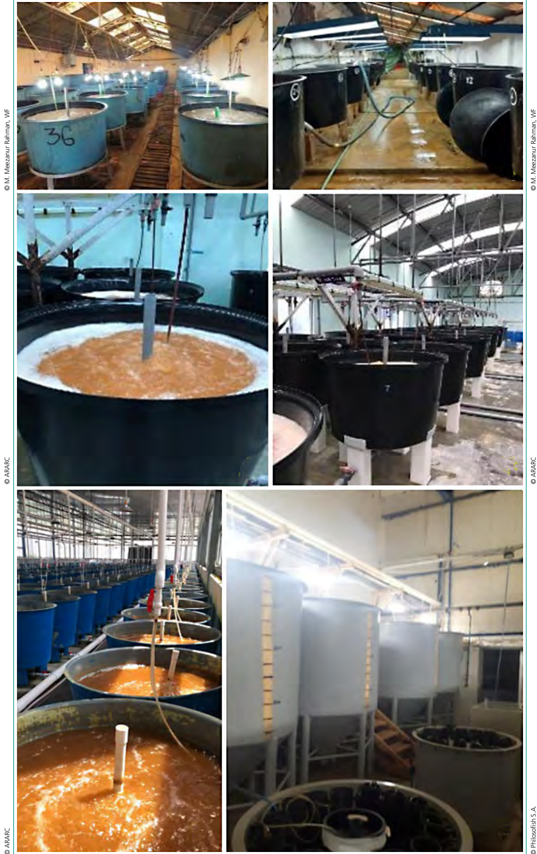
PLATE 54 Different types and sizes of cylindroconical hatching tanks in different hatcheries around the world, from small conical tanks of a few 100 L up to 2 500 L
